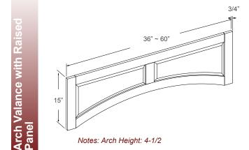
Weight Item Code Dimensions RPV36-A 36W x 15H x 3/4D 7 LB 42W x 15H x 3/4D 8 LB RPV42-A 48W x 15H x 3/4D RPV48-A 9 LB RPV54-A 54W x 15H x 3/4D 10 LB RPV60-A 60W x 15H x 3/4D 11 LB
